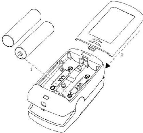
**Figure 3 Battery Installation**
